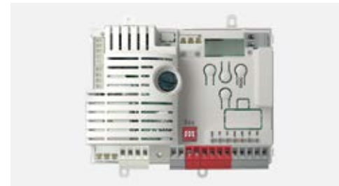
New control unit CT10324 with integrated receiver programmable with KUBEPRO
